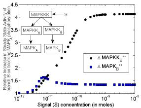
**Figure 4:** The relative increase in the response of branch B as a function of signal strength, when the phosphorylation of MAPK in branch A is inhibited by an ATP blocker. The increase is measured as the ratio of steady-state concentrations for MAPK<sub>B</sub>\*\* and MAPK<sub>B</sub>\*\* on inhibiting branch A to their concentrations under normal conditions. The inset shows a schematic diagram of the branched MAPK reaction network.
