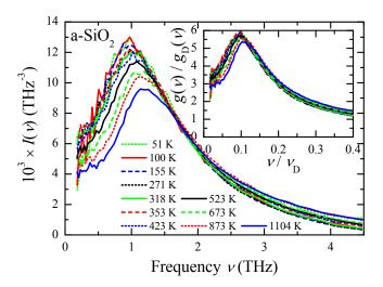
FIG. 2: The neutron scattering BP of silica at 11 different temperatures. The Debye level at 1 THz calculated from the velocity in Fig. 1c is already subtracted. The inset illustrates a scaling of the entire  $g(\nu)$  using the Debye frequency at 1 THz, the BP frequency.
