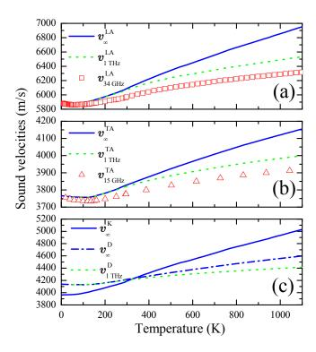
FIG. 1: The T-dependence of the sound velocities measured in silica with Brillouin scattering (points) and renormalized to 1 THz (dashed lines) and to infinite frequency (solid lines): (a) the LA mode; (b) the TA mode; (c) the calculated Debye velocities  $v^{\rm D}$  at two frequencies compared to the bare bulk-modulus "velocity"  $v_{\infty}^{\rm K}$ .
