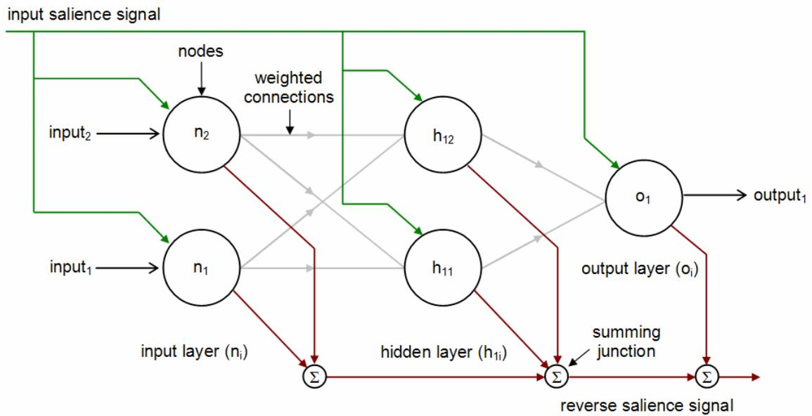
Figure 1: An SANN with a 2-node input layer ( $n_i$ ), a 2-node hidden layer ( $h_{i_i}$ ), and a single output node ( $o_i$ ). Each node receives an *input salience signal*, which has the effect of varying the threshold value of the sigmoidal function at each individual node, during training, depending on the node's activation level. From each node, *nodal reverse salience signals* are summed, to create a *reverse salience signal* for the SANN.
