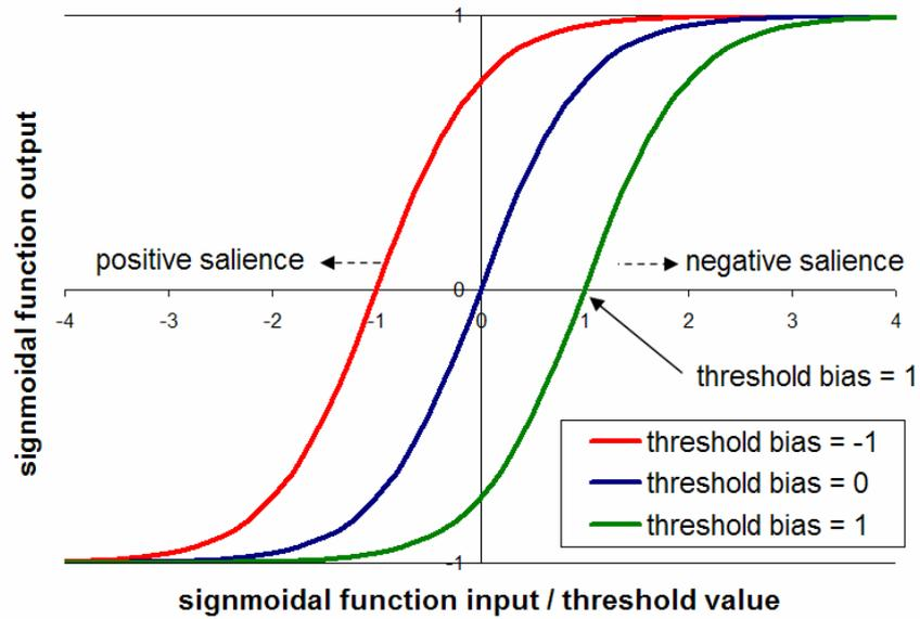
Figure 2: Varying thresholds of an approximate *tanh*-based sigmoidal function. It can be seen that the input salience signal applied to each node has the effect of pushing active node's threshold closer to their activation threshold (for positive salience), or moving them further away from this threshold (for negative salience).
