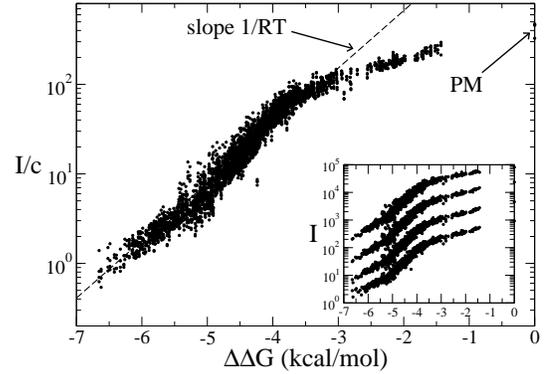
FIG. 1: Plot of  $I/c$  as a function of  $\Delta\Delta G$  for four different experiments at concentrations  $c = 2, 10, 50$  and  $250$  pM. The hybridization time is of 17 h. The “collapse” of the four data sets into a single curve demonstrates that  $I \propto c$  in the whole intensity range. Deviations from the equilibrium isotherm  $I \propto e^{-\Delta G/RT}$  are observed at high intensities. Inset: plot of each individual concentration.
