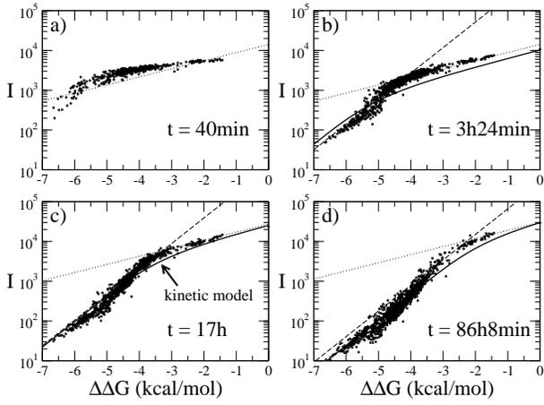
FIG. 2: Plot of intensity vs.  $\Delta\Delta G$  four experiments at different times with a 30-mer target and  $c = 50$  pM. Dashed lines have slope  $1/RT$ , dotted lines have slope  $\gamma/RT$  with  $\gamma = 0.32$ . Solid lines are obtained from the solution of Eqs. (2) and (3) using as parameters  $k_1 = 10^5 M^{-1} s^{-1}$ ,  $k_2 = 1 s^{-1}$ ,  $\gamma = 0.32$  and  $\Delta G_{PM} = -14.5$  kcal/mol.
