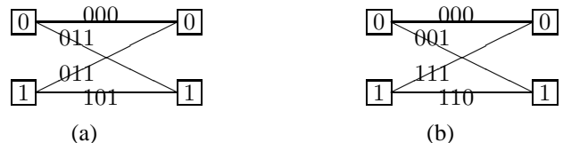
Fig. 4. Trellis sections of (a) rate-1/3 2-state binary convolutional code \mathcal{C}_1 ; (b) similar code \mathcal{C}_2 .
