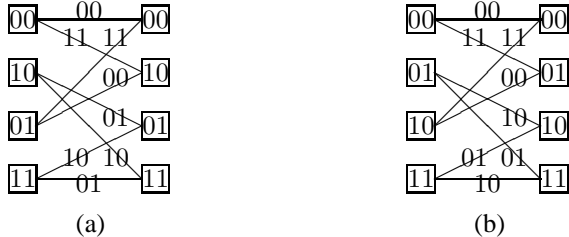
Fig. 1. Trellis sections of (a) rate-1/2 4-state binary convolutional code \mathcal{C} ; (b) orthogonal code \mathcal{C}^\perp .
