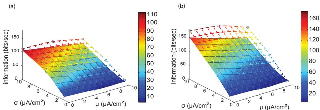
FIG. 8: (Color online) Difference between Langevin and Markov models of channel noise with 2 levels of input noise for a  $10 \mu m^2$  compartment ( $f_c = 300 Hz$ ). Filled mesh represents the Markov model, wireframe mesh displays the Langevin model.  $\mu$  is the mean and  $\sigma$  is the standard deviation of the current injection. (a): Signal-to-noise ratio equals 2, (b): Signal-to-noise ratio equals 20.
