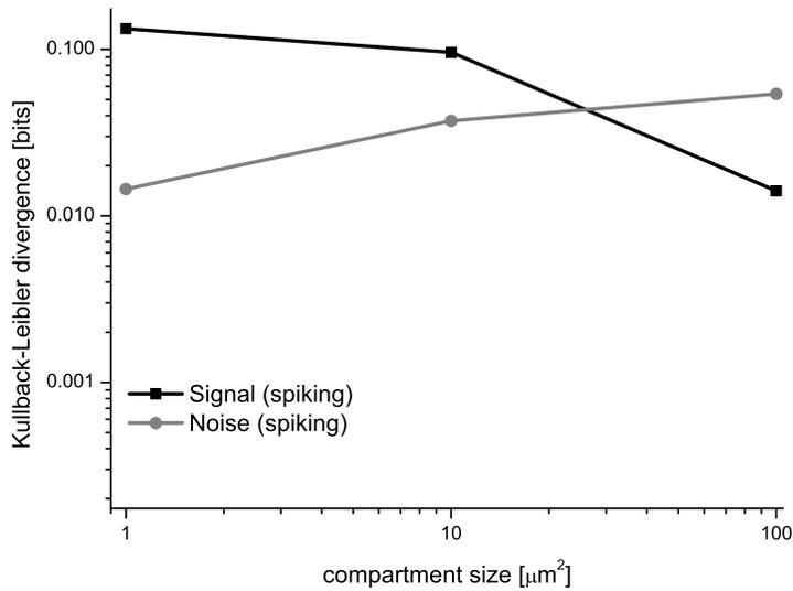
FIG. 7: (Color online) Comparison of probability density function of Langevin and Markov models of channel noise for spiking compartments. The distance between the distributions is quantified by the Kullback-Leibler (relative entropy) divergence. Input statistics were sampled from a Gaussian distribution with  $\mu = 5 \mu A/cm^2$ ,  $\sigma = 10 \mu A/cm^2$  and  $\tau_{correlation} = 3.3 ms$ .
