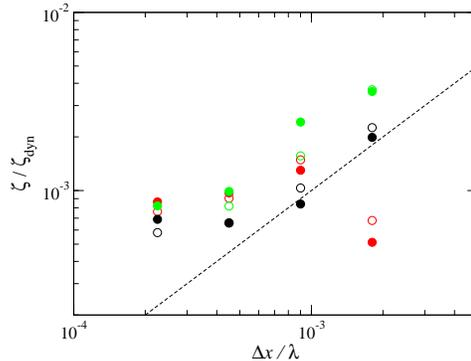
**Figure 3.** Dependence of the numerical viscosity  $\zeta$  on the resolution in neutron star evolution. We show values for different flux formulae, Marquina (filled circles) and HLL (open circles), and different reconstruction schemes, constant (black), minmod (red) and MC (green). In all cases the highest metric resolution case is plotted. The dashed line represents the function  $\zeta/\zeta_{\text{dyn}} = \Delta r/\lambda$ .
