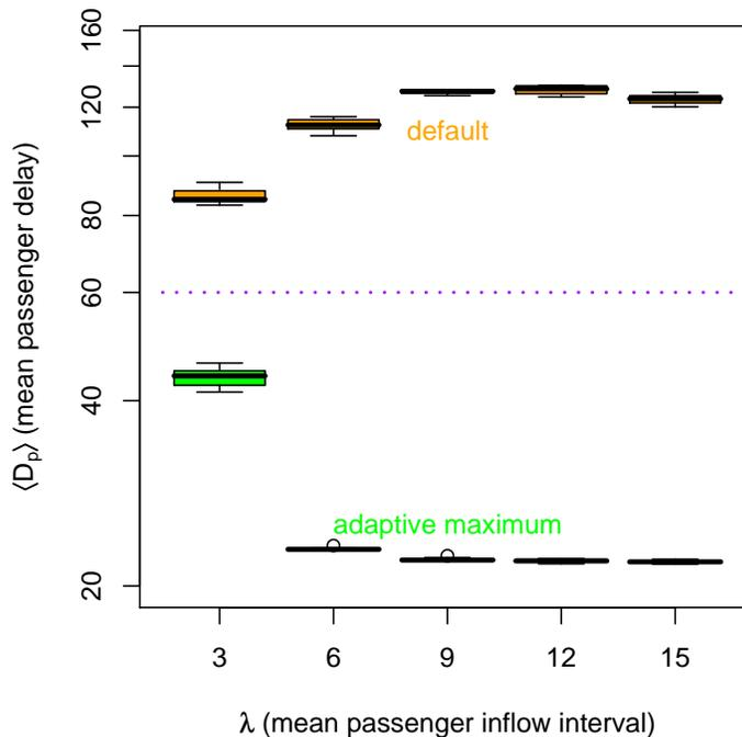
Figure 4: Comparison of passenger delays  $D_p$  between *default* and *adaptive maximum* methods, varying mean passenger inflow intervals  $\lambda$ . For  $\lambda > 3$ , the mean delays for the *default* method are about six times larger than those for the *adaptive maximum* method (notice logarithmic scale on  $y$  axis).
