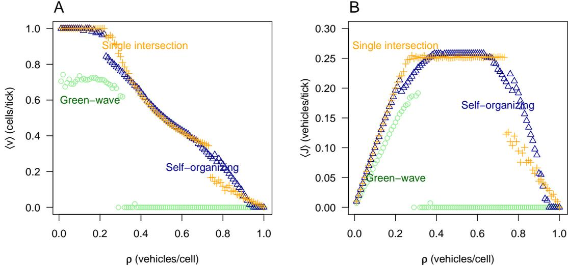
Figure 2: Simulation results for a ten-by-ten city grid: (A) average velocity  $\langle v \rangle$  and (B) average flux  $\langle J \rangle$  for different densities  $\rho$ , *green-wave* (O) and *self-organizing* ( $\Delta$ ) methods. For comparison, results for a single intersection (+) are also shown.
