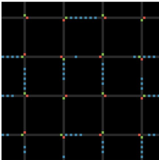
Figure 1: Screenshot of the simulation. With the *self-organizing method*, free flow is achieved in four directions for low densities ( $\rho = 0.1$  shown), as vehicles trigger green lights before reaching intersections.
