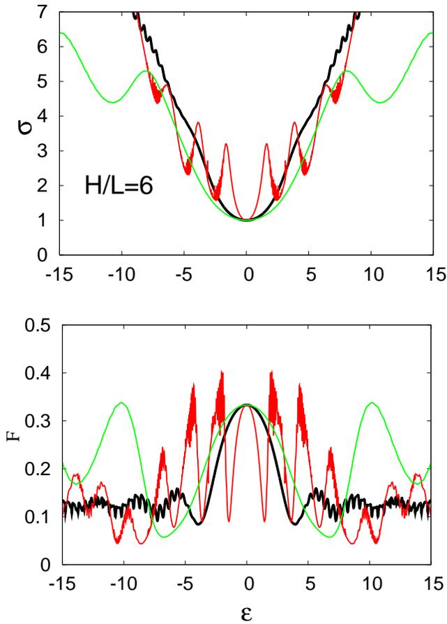
FIG. 5: Conductivity  $\sigma$  in units of  $2e^2/h$  and Fano factor  $F$  as a function of the energy of the incoming Dirac fermions: Green, Red, and black correspond to  $v_F$  5, 0.2, and 1.0 respectively.  $\epsilon$  is  $eVH/hv_F$  where  $V$  is the gate voltage.
