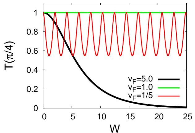
FIG. 4: (Color online). Transmission probability as a function of the width  $W$  for fixed energy  $E_F = 100$  meV and angle  $\phi = \pi/4$ . Curves in green, red, and black correspond to velocities  $v_F = 1, 1/5$ , and  $5$ , respectively, inside the barrier.
