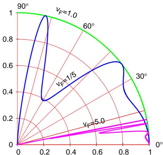
FIG. 3: (Color online). Transmission probability at  $E_F = 100$  meV,  $W = 350$  nm and velocities inside the barrier  $v_F = 1, 1/5$ , and  $5$  (green, blue, and pink lines respectively). Resonances are apparent at  $Wq_x = n\pi$ , with  $n = 0, 1, 2, \dots$ . Note that for  $v_F > 1$  no transmission is allowed if  $\phi > \phi_{cr}$ .
