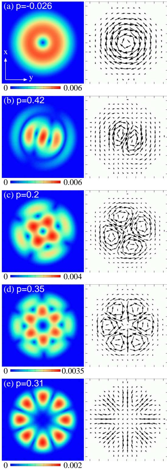
FIG. 3: (color) Magnitude of the integrated transverse magnetization  $|\int F_+ dz|$  (right panels) and its direction  $\arg(\int F_+ dz)$  (left panels) at the first peaks of the curves in Fig. 2. The values of  $p \equiv (P - Q)/(\hbar\omega_\perp)$  used are indicated by the arrows in Fig. 1. The unit of  $\int F_+ dz$  is  $NM\omega_\perp/\hbar$ . The length of the vector is proportional to  $|\int F_+ dz|$ . The field of view is  $9.7 \times 9.7 \mu\text{m}$ .
