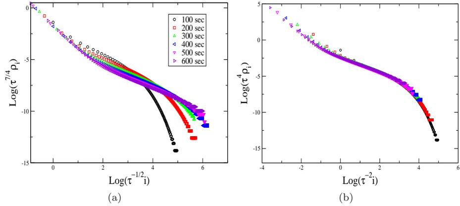
FIG. 4: (a) Scaling collapse for the intermediate bundle sizes with  $\sigma = 10 \text{ nM}$ ,  $\theta_c = 20^\circ$ , and  $\rho_m = 10 \mu\text{M}$ . The curves clearly illustrate convergence towards the proposed scaling in this region. (b) Scaling collapse for large bundle sizes with  $\sigma = 10 \text{ nM}$ ,  $\theta_c = 20^\circ$ , and  $\rho_m = 10 \mu\text{M}$ .
