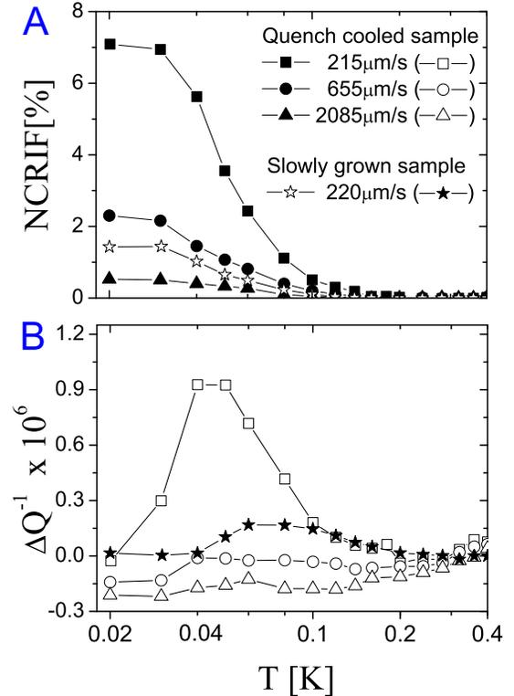
FIG. 1: Non-classical rotational inertia fraction (A) and dissipation (B) of the quench-cooled solid  $^4\text{He}$  in porous gold. The symbol with the open star (solid star) represents the NCRI (dissipation) of the slow-cooled sample.
