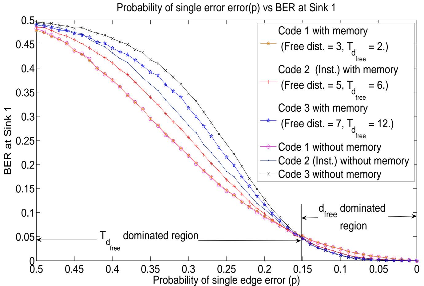
Fig. 14. BER (with and without memory) at Sink 1
