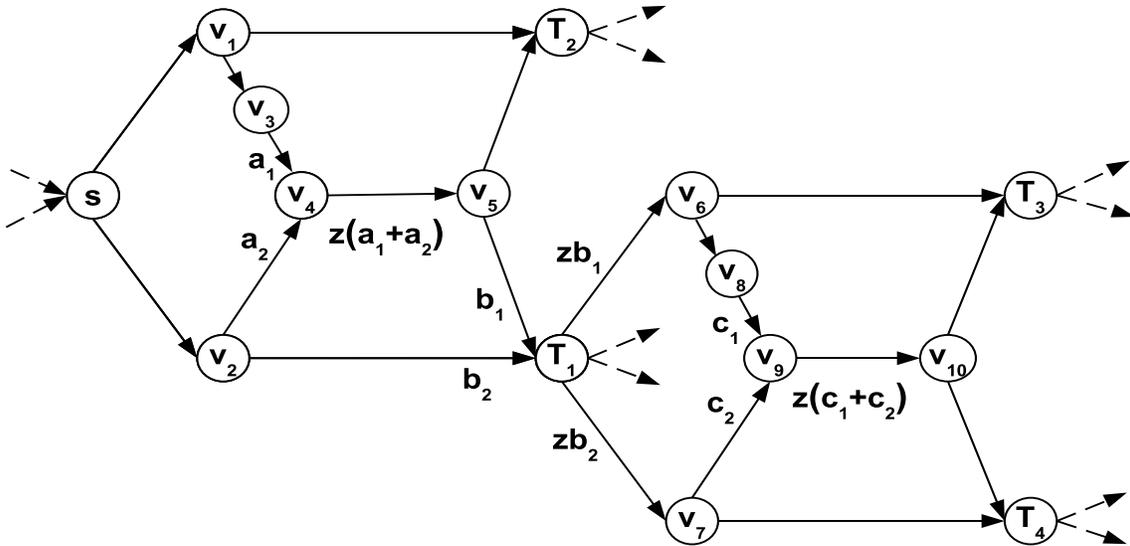
Fig. 9. Figure corresponding to Example 9. A modified double-butterfly network. The mapping between the incoming and outgoing symbols ( $a_1, a_2, b_1, b_2, c_1, c_2 \in \mathbb{F}_2$ ) at the nodes  $v_4, T_1$ , and  $v_9$  are shown.
