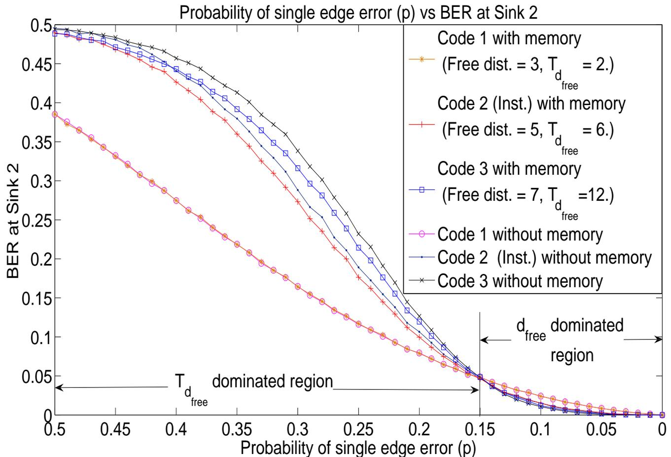
Fig. 15. BER (with and without memory) at Sink 2
