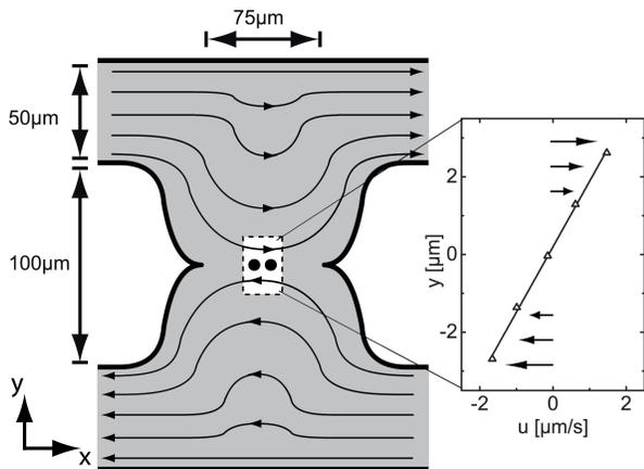
FIG. 1: A cell cross-section (lithographic mask) is shown with  $150\mu\text{m}$  depth in the  $z$  direction having opposite flow directions in its upper and lower channel and a linear shear profile at its center: see inset with PIV data ( $\Delta$ ) and linear fit. One or two particles at a distance  $d = 4\mu\text{m}$  were held by optical tweezers in the center of the linear velocity profile  $\mathbf{u}(y)$ .
