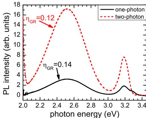
FIG. 8: (Color online) Time-integrated photoluminescence of annealed ZnO under one-photon and two-photon excitation.
