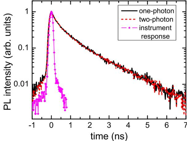
FIG. 5: (Color online) Time-resolved photoluminescence of unannealed ZnO under one-photon and two-photon excitation. The corresponding window of spectral integration was centered at the X-2LO transition ( $3.177 \text{ eV} \pm 0.036 \text{ eV}$ ).
