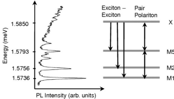
**FIG. 2.** Below threshold photoluminescence spectrum from a  $3.2\mu\text{m}$  square pillar at  $\delta = -13$  meV detuning and schematic representation of the energy transitions between the exciton reservoir and polariton states M1, M2 and M5. Arrows indicate exciton-exciton and pair-polariton scattering between the states.
