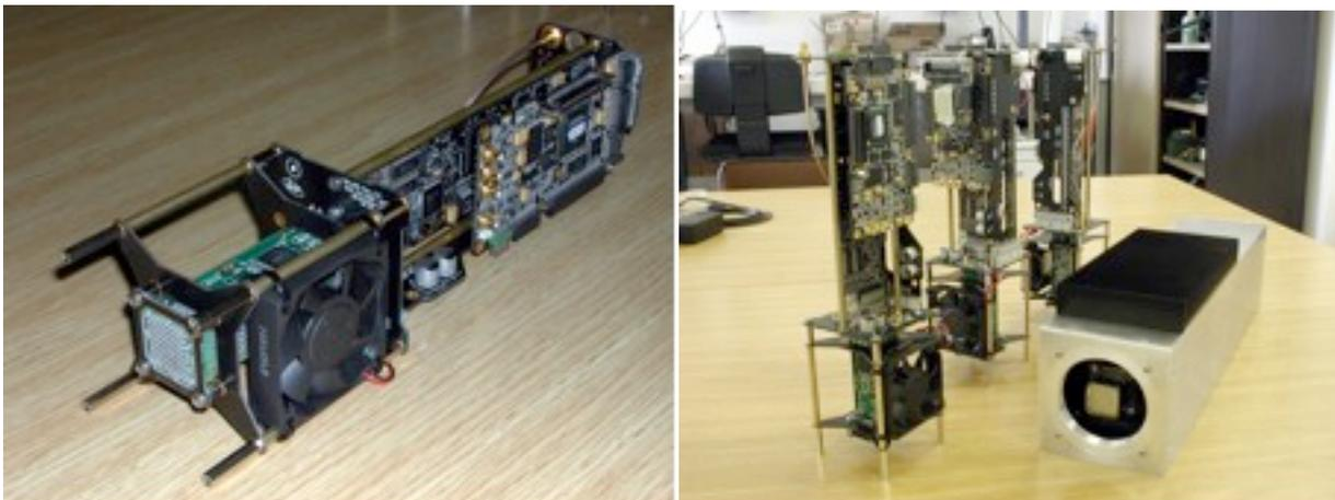
Fig. 5.4.2: (left panel) is shown an apparatus, realized in IASF-Palermo, to test and qualify MAPT Hamamatsu R7600, GAW experiment [12]. Right panel shows the apparatus within its mechanical box.
