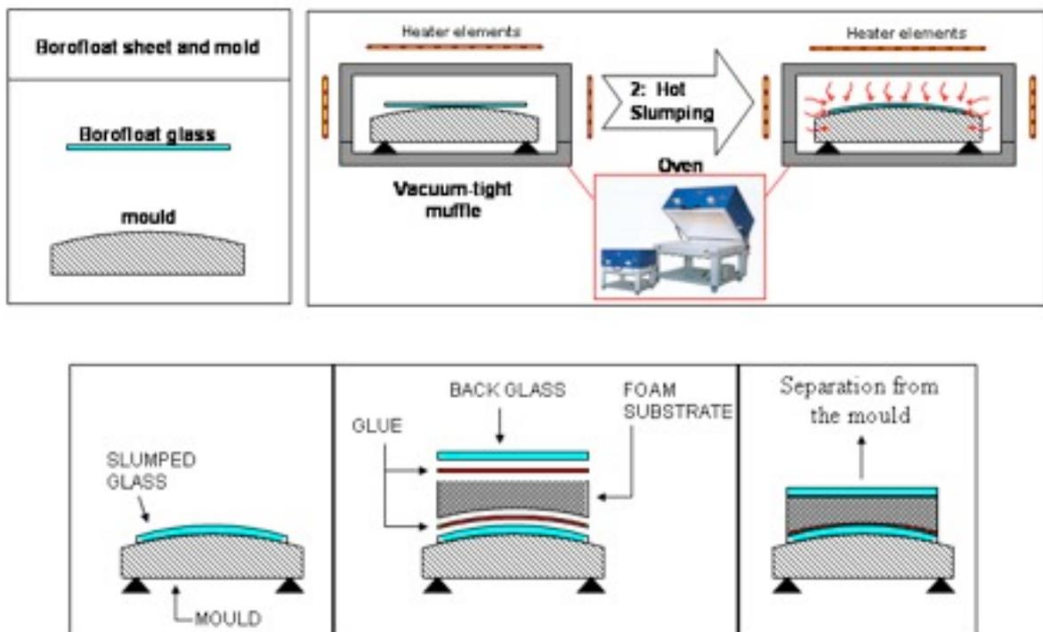
Fig. 5.3.2: Hot slumping technique for the production of optical panels.
