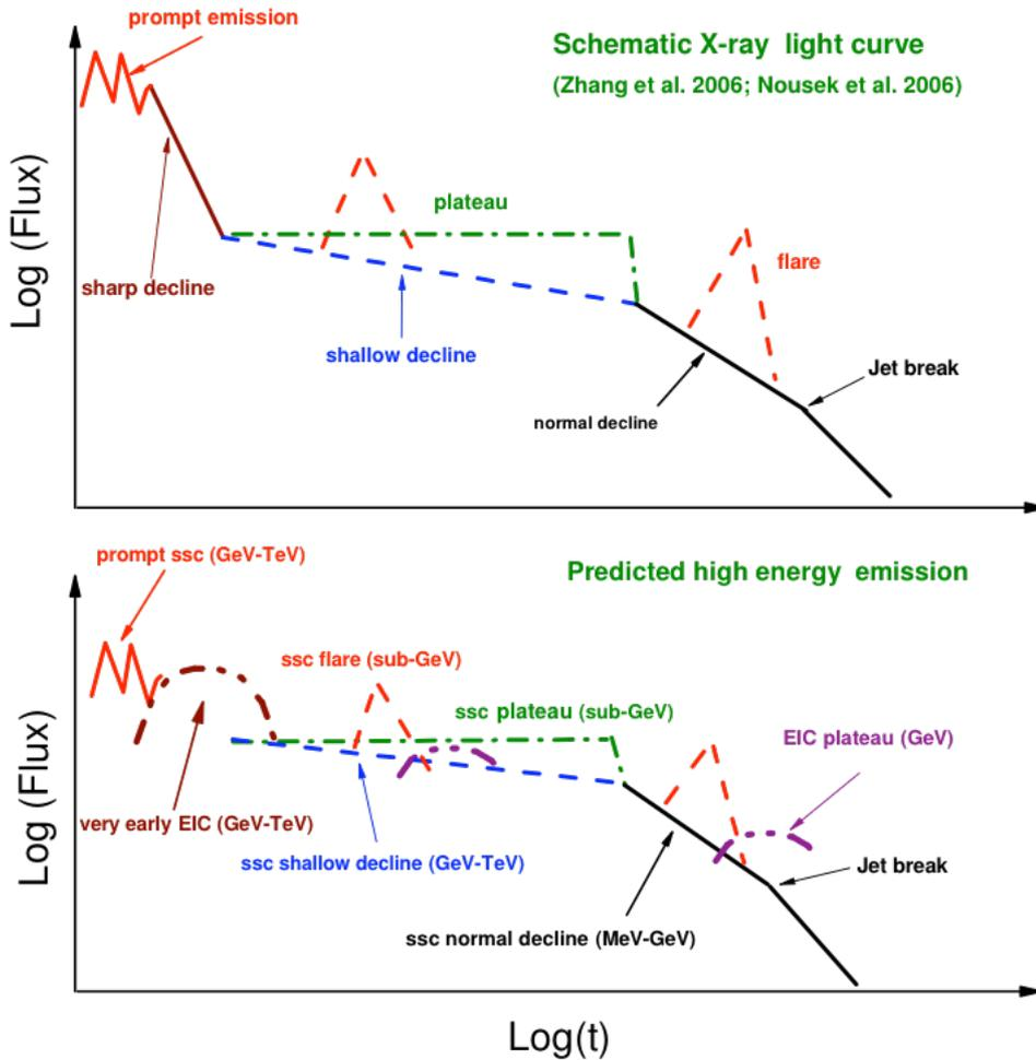
**Fig. 3.4.1:** Schematic view of the typical soft-X-ray light curve for a GRB and possible high-energy processes shaping the higher energy light-curve (from [41]).
