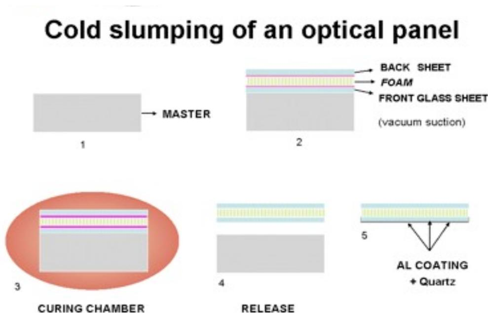
Fig. 5.3.1: Cold slumping technique for the production of optical panels.
