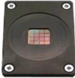
**Fig. 5.4.4:** SiPMArray constituted by 4 x 4 SiPM of 3x3 mm<sup>2</sup> (Position Sensitive Multi Anode High Gain APDS).
