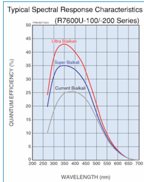
Fig. 5.4.1: Spectral Response for Super and Ultra Bialkali photo cathodes in MAPT Hamamatsu R7600 [11].
