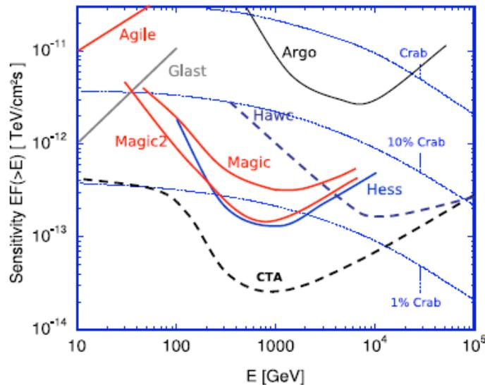
**Fig. 5.1:** Sensitivities of some present and future HE gamma detector, measured as the minimum intensity source detectable at 5 sigma [1]. The performance for EAS and satellite detector is based on one year of data taking; for Cherenkov telescopes it is based on 50 hours of data.
