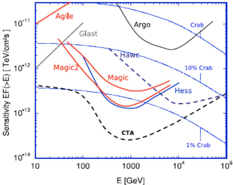
**Fig. 1.4.1:** Sensitivities of some present and future HE gamma detector, measured as the minimum intensity source detectable at 5 sigma. The performance for EAS and satellite detector is based on one year of data taking; for Cherenkov telescopes it is based on 50 hours of data (from [3]).
