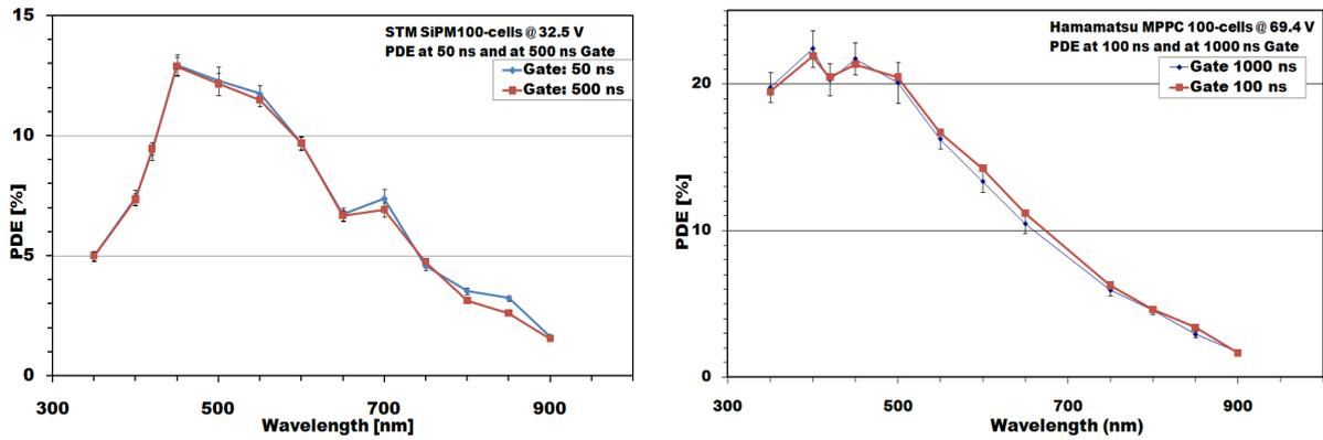
**Fig. 5.4.6:** (Left panel) The PDE of the STM device biased at 32.5 V. (Right panel) The PDE measured for the Hamamatsu 100 cells biased at 69.4 V.
