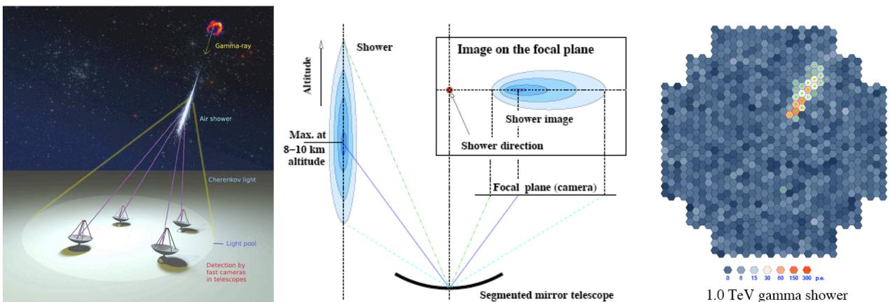
**Fig 1.2.2:** *Left:* Schematic of the Cherenkov light pool, originating from a primary  $\gamma$ -ray and illuminating an array of telescopes. *Central:* Shower imaged by a telescope. The shower image in the camera has an elliptical shape and the shower direction lays on the extension of its major axis; the image intensity is related to the primary energy. *Right:* Image of a  $\gamma$ -induced air shower in the camera. (From [2])
