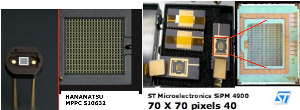
**Fig. 5.4.5:** (Left panel) 100-cells Hamamatsu Multi Pixel Photon Counter (MPPC) device. (Right panel) 100-cells STM SiPM device. Both sensors have been operated using a bias over-voltage of about 10% for the STM (breakdown voltage is about 29.5 Volts) and of about few percent for the Hamamatsu (breakdown voltage is about 68,6 V).
