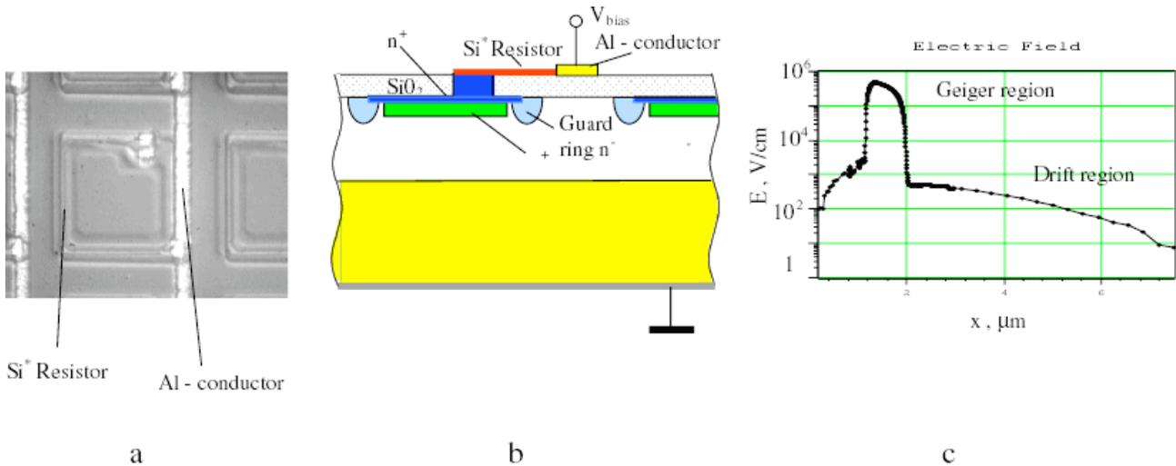
**Fig. 5.4.3:** (a) SEM microphotography of a SiPM micro-pixel, (b) schematic section of the micro-pixel (c) electric field dependence through a vertical section of the micro-pixel.
