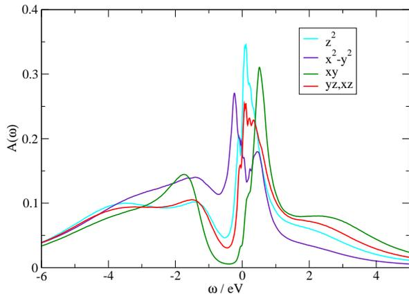
FIG. 6: (Color online) Impurity spectral function within the  $d$  hamiltonian using interaction parameters  $U = 4.0$  eV and  $J = 0.7$  eV as have been used in Ref. 2. For those values a very correlated metal is obtained.
