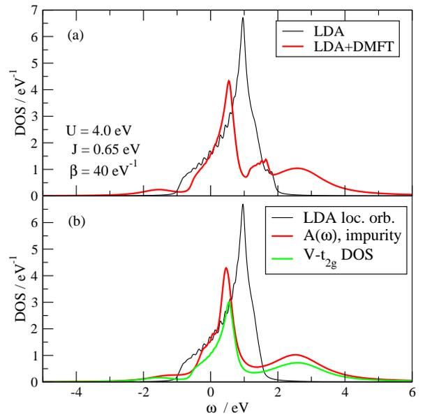
FIG. 7: (Colore online) DOS for SrVO<sub>3</sub>,  $d$ -only model (small energy window). Top panel (a): Total DOS of LDA (black) and LDA+DMFT (red). Bottom panel (b): LDA local orbitals (black), impurity spectral function  $A(\omega)$  (red), and vanadium  $\hat{2}g$  partial DOS (green). Coulomb parameters for these calculations are given as inset.
