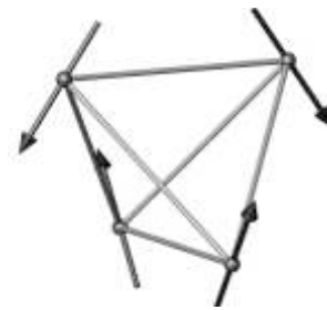
FIG. 13 Ground state spin configuration determined for \text{Er}_2\text{Ti}_2\text{O}_7 (Poole et al. , 2007). In a macroscopic sample six symmetry equivalent spin configurations will co-exist.
