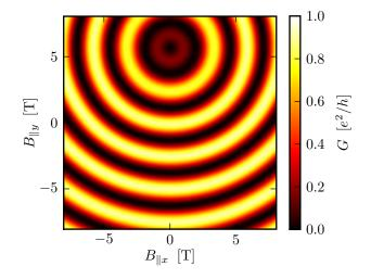
FIG. 2: Dependence of the conductance of the HgTe quantum well on the parallel magnetic field  $B_{\parallel}$ , calculated from the tight-binding model for  $B_{\perp} = B_c = 6.09 \text{ T}$ .
