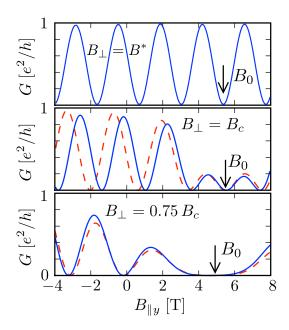
FIG. 3: Dependence of the conductance on  $B_{\parallel y}$  for  $B_{\parallel x} = 0$ , at three values of the perpendicular magnetic field. The solid curves are calculated numerically from the tight-binding model, the dashed curves are the analytical prediction (16). The arrow indicates the value of  $B_0$  from Eq. (17). (Only the numerical curve is shown in the upper panel, because the analytical curve is nearly indistinguishable from it.)
