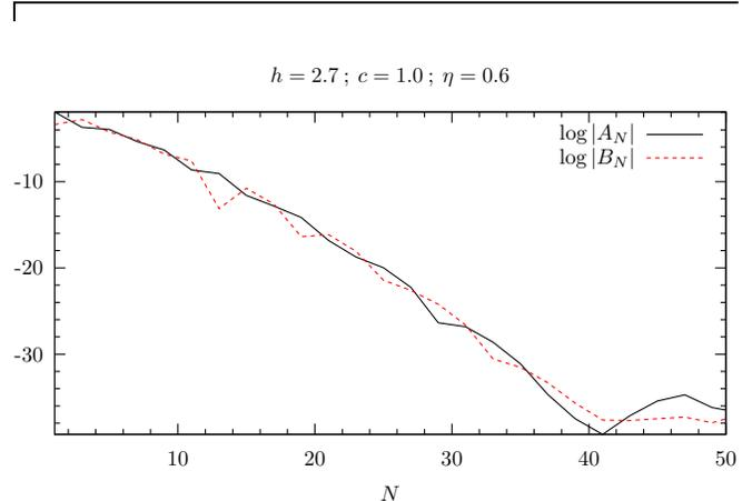
FIG. 6: Plotting the logarithms of  $|A_N|$  and  $|B_N|$  reveals the exponential decay with  $N$ . In the regime where numerical errors do not dominate the result, a linear regression seems appropriate.
