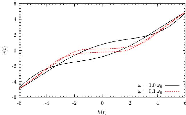
FIG. 3: Numerical solution of equation (47) for  $h = 6.0$ ,  $c = 1.0$  and  $\eta = 2.5$  for different frequencies,  $t$  and  $z$  being measured in units such that  $\omega_0 = \ell = 1$ .
