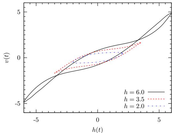
FIG. 2: Numerical solution of (47) for different driving field strengths and  $c = 1.0$ ,  $\eta = 2.5$ . For the simulation,  $t$  and  $z$  are measured in units such that  $\omega = \ell = 1$ .
