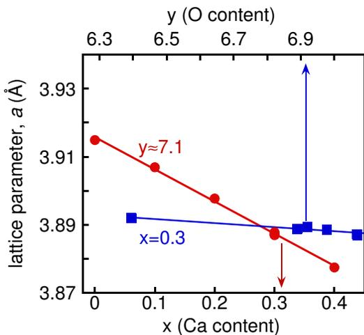
FIG. 4: (Color online) In plane lattice parameter  $a$  of  $\text{Ca}_x\text{La}_{1-x}\text{Ba}_{1.75-x}\text{La}_{1.25+x}\text{Cu}_3\text{O}_{6+y}$  at  $y \sim 7.13$  vs. calcium content (bottom axis), and at  $x = 0.3$  vs. oxygen content (top axis). The lattice parameter  $a$ , which is directly related with the chemical pressure on the  $\text{CuO}_2$  layers, changes as the Ca concentration is modified, while remains nearly constant as oxygen is introduced.
