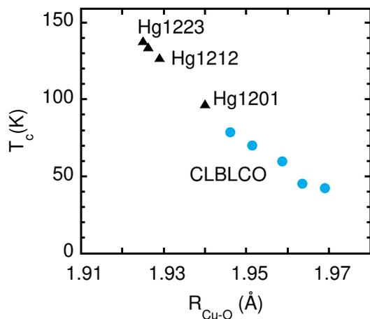
FIG. 5: (Color online)  $T_c^{max}$  as a function of the Cu-O inplane distance,  $R_{\text{Cu-O}} = a/(2\cos\theta)$  (where  $\theta$  is the buckling angle of the  $\text{CuO}_2$  planes). The data for the Hg-cuprate family are from Ref.<sup>29</sup>.
