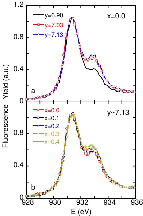
FIG. 1: (Color online) Comparison of the Cu L edge XAS spectra of  $\text{Ca}_x\text{La}_{1-x}\text{Ba}_{1.75-x}\text{La}_{1.25+x}\text{Cu}_3\text{O}_{6+y}$ , measured at  $T=20$  K, for various O contents,  $y$ , (upper panel) and Ca concentrations,  $x$  (lower panel). The introduction of oxygen produces an increase of the intensity of the feature at 933 eV (ligand holes). Negligible variations are observed in the spectra as a function of Ca concentration.
