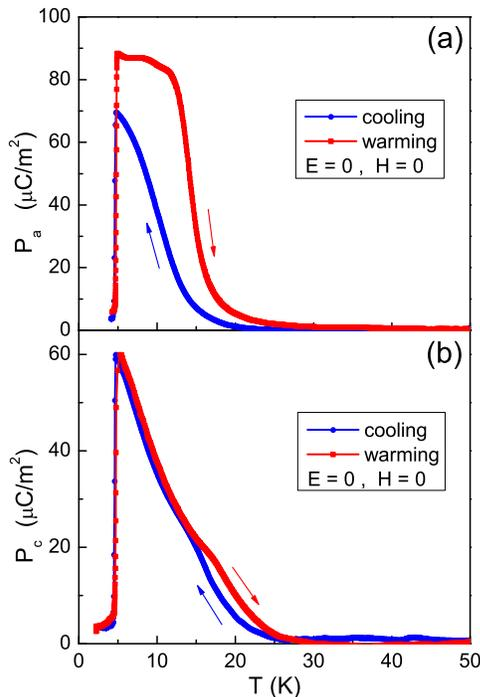
FIG. 6: (Color online) Polarization of  $\text{HoFe}_3(\text{BO}_3)_4$  measured along (a): the a-axis and (b): the c-axis in zero electric and magnetic fields. The arrows distinguish the cooling and warming data.
