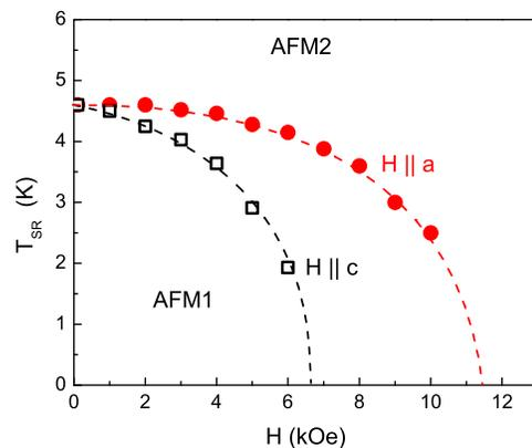
FIG. 3: (Color online) Low-temperature  $T$ - $H$  phase diagram of  $\text{HoFe}_3(\text{BO}_3)_4$  with the field aligned with the  $a$ -axis (bold symbols) and the  $c$ -axis (open symbols). The lines serve as a guide to the eye.
