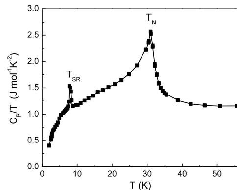
FIG. 13: Heat capacity of  $\text{Ho}_{0.5}\text{Nd}_{0.5}\text{Fe}_3(\text{BO}_3)_4$ .
