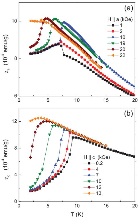
FIG. 11: (Color online) Magnetic susceptibility of  $\text{Ho}_{0.5}\text{Nd}_{0.5}\text{Fe}_3(\text{BO}_3)_4$  at low temperatures in different magnetic fields. (a):  $H \parallel a$ -axis and (b):  $H \parallel c$ -axis.
