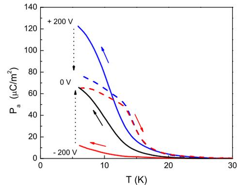
FIG. 7: (Color online) a-axis polarization of  $\text{HoFe}_3(\text{BO}_3)_4$  measured upon cooling (solid lines) with applied bias voltage of +200 V, 0 V, and -200 V. Data upon warming (dashed lines) are collected after release of the bias voltage at 6 K.
