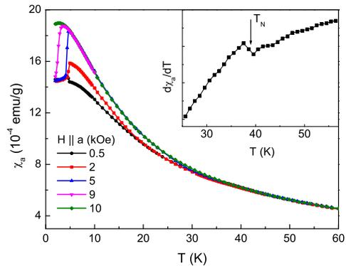
FIG. 1: (Color online) Magnetic susceptibility of  $\text{HoFe}_3(\text{BO}_3)_4$  with the field oriented along the a-axis. The inset shows the derivative,  $d\chi_a/dT$ , with the distinct anomaly at  $T_N$ .
