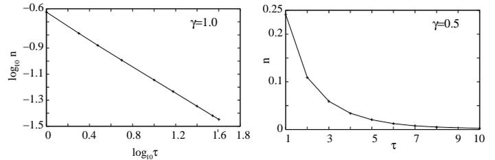
FIG. 2: Numerical integration result for the defect density as a function of  $\tau$  for  $\gamma = 1$  and  $\gamma = 0.5$ . The parameter  $\alpha$  is chosen such that the system crosses both the gapless phases in the two cases. For  $\gamma = 1$ , we have used log-scale and slope of the straight line is  $1/2$  indicating a power-law decay of the defect density. For  $\gamma = 0.5$ , we have used linear scale to accentuate the exponential fall of the defect density.
