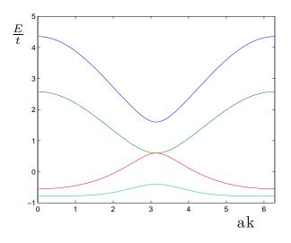
FIG. 3: An exemplifying image for the band structure plotted on a  $2\pi$  domain for the k variable. The used parameters are  $t_1/t = 1, t'/t = 0.2, t'_1/t = 0.2, t_e/t = 0.2, \epsilon_0/t = 1, \epsilon_1/t = 1$ . By modifying the  $\hat{H}_0$  parameter values and signs, the relative inter-band distances and band shapes can be changed.
