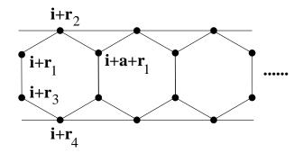
FIG. 1: The studied zig-zag hexagon chain. The cell constructed at the site **i** contains 4 sites whose in-cell positions relative to **i** are specified by the vectors  $\mathbf{r}_{\nu}$ ,  $\nu = 1, 2, 3, 4$ , where, for convenience one takes  $\mathbf{r}_1 = 0$ . The vector **a** represents the unique primitive vector of the Bravais lattice. In the same time,  $\mathbf{r}_{\nu}$  denotes lattice sites in four different sublattices  $S_{\nu}$ .
