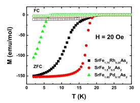
FIG. 4: (Color online) Temperature dependence of DC magnetization for the samples  $SrFe_{1.75}Rh_{0.25}As_2$ ,  $SrFe_{1.5}Ir_{0.5}As_2$  and  $SrFe_{1.85}Pd_{0.15}As_2$ . The measurement was done under a magnetic field of 20 Oe with zero-field-cooled and field-cooled modes. Strong diamagnetic signals were observed here.
