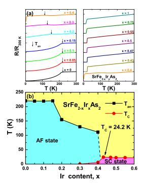
FIG. 6: (Color online) (a) Temperature dependence of resistivity and (b) phase diagram for compounds  $SrFe_{2-x}Ir_xAs_2$  with the Ir content x from 0 to 1. The antiferromagnetic order of the parent phase begins to be suppressed at x=0.2. The superconductivity starts to appear at x=0.4, and reaches a maximum  $T_c$  of 24.2 K rapidly at about x=0.43.
