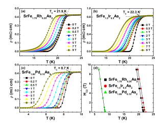
FIG. 8: (Color online) Temperature dependence of resistivity for the samples (a)  $SrFe_{1.75}Rh_{0.25}As_2$ , (b)  $SrFe_{1.5}Ir_{0.5}As_2$ , and (c)  $SrFe_{1.85}Pd_{0.15}As_2$  at different magnetic fields. The dashed line indicates the extrapolated resistivity in the normal state. One can see that the superconductivity seems to be robust against the magnetic field and shifts slowly to the lower temperatures. (d) The upper critical field determined using the criterion of  $90\%\rho_n$ .
