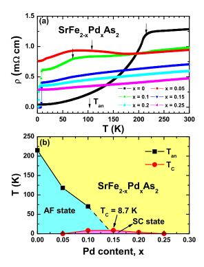
FIG. 7: (Color online) (a) Temperature dependence of resistivity and (b) phase diagram for compounds  $SrFe_{2-x}Pd_xAs_2$  with the Pd content x ranging from 0 to 0.25. The superconductivity starts to appear at x=0.1, reaching a maximum  $T_c$  of 8.7 K at x=0.15.
