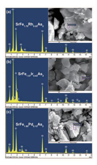
FIG. 3: (Color online) The Energy dispersive X-ray microanalysis (EDX) spectrums of the the samples (a)  $SrFe_{1.75}Rh_{0.25}As_2$ , (b)  $SrFe_{1.57}Ir_{0.43}As_2$  and (c)  $SrFe_{1.85}Pd_{0.15}As_2$ . The spectrums are taken from the main grains and show that the main elements of the grains are Sr, Fe, M (M = Rh, Ir and Pd, respectively) and As. The insets show the scanning electron microscopic pictures. The little rectangles mark the positions where we took the EDX spectrums.
