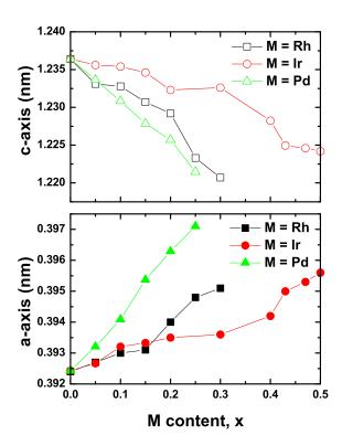
FIG. 2: (Color online) Doping dependence of the c-axis lattice constant (top panel) and a-axis lattice constant (bottom panel). It shows a common feature that the a-axis lattice constant expands, while the c-axis one shrinks monotonically with Rh, Ir and Pd substitution. This systematic evolution clearly indicates that the Rh, Ir and Pd ions have been successfully substituted into the Fe-sites. The x here represents the nominal concentration of the dopants.
