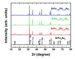
FIG. 1: (Color online) X-ray diffraction patterns of the samples SrFe<sub>2</sub>As<sub>2</sub>, SrFe<sub>1.75</sub>Rh<sub>0.25</sub>As<sub>2</sub>, SrFe<sub>1.57</sub>Ir<sub>0.43</sub>As<sub>2</sub> and SrFe<sub>1.85</sub>Pd<sub>0.15</sub>As<sub>2</sub>. The latter three samples have the optimized superconducting transition temperatures in their own phase diagrams as shown below. Almost all main peaks can be indexed by a tetragonal structure and the impurity phases are negligible.
