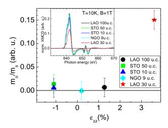
Figure 7: (Color online) Orbital to spin moment ratio as a function of the out-of-plane strain for all investigated LSMO films on STO, NGO and LAO substrates. The corresponding XMCD spectra, normalized to the sum of the XAS  $L_3$  peak height signals, are reported in the inset.
