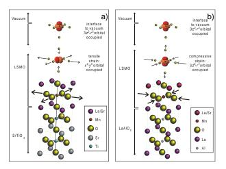
Figure 1: (Color online) Schematics of the influence of strain onto the orbital occupation in the bulk and at the interface of LSMO films. The bulk Mn 3d orbital occupation is  $x^2 - y^2$  and  $3z^2 - r^2$  in case of SrTiO<sub>3</sub> (a) and LaAlO<sub>3</sub> (b) substrate respectively. The preferential orbital occupation is  $3z^2 - r^2$  at both interfaces.
