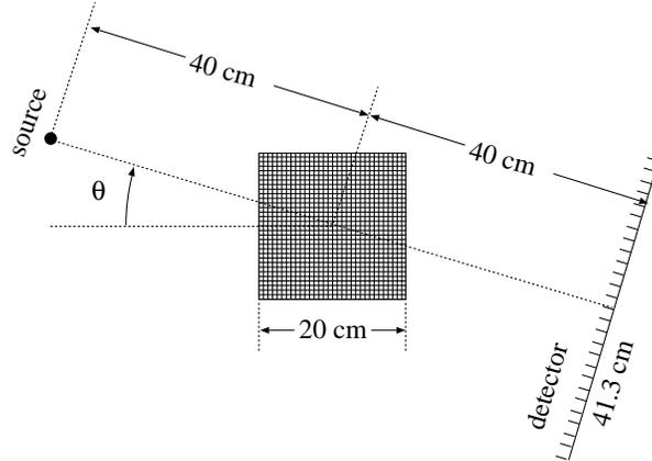
FIG. 2: Fan-beam CT configuration used in the simulations presented in this work. The 256x256 image array is 20x20 cm<sup>2</sup>, and the detector is composed of 512 bins. The center of rotation for the source-detector gantry coincides with the center of the image array.
