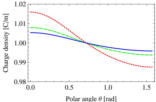
FIG. 2: Approach of the linear charge density to uniformity for an elliptical filament. The three graphs show the charge density for the first quadrant of the elliptical filament, at  $\epsilon = 10^{-4}$  (short dash, red),  $\epsilon = 10^{-8}$  (long dash, green), and  $\epsilon = 10^{-12}$  (solid, blue). Note the logarithmically slow rate of convergence to uniformity.
