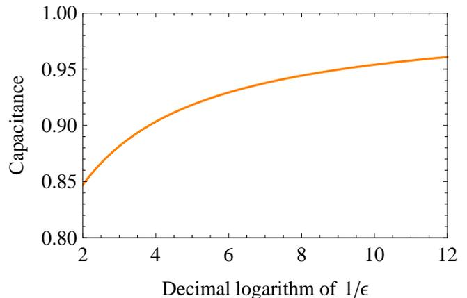
FIG. 4: Capacitance per unit length of an elliptical filament relative to a circular one as its diameter shrinks by 10 orders of magnitude; see text.
