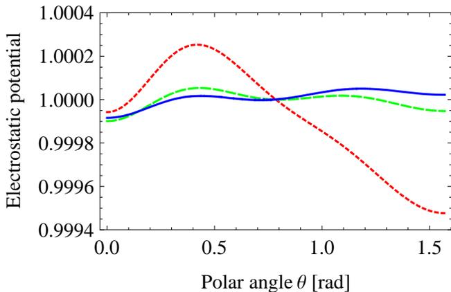
FIG. 3: Approach of the electrostatic potential to uniformity for an elliptical filament. The three graphs show the electrostatic potential, normalized to unity at  $\theta = \pi/4$ , for the first quadrant of the elliptical filament, at  $\epsilon = 10^{-4}$  (short dash, red),  $\epsilon = 10^{-8}$  (long dash, green), and  $\epsilon = 10^{-12}$  (solid, blue).
