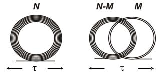
FIG. 9: Sketch of N, N-M and M tori. Physically we expect the energy barrier between these to be dependent only on surface energy difference, as the bending energy and tension are unchanged.
