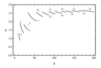
FIG. 5: Tension vs reduced length for preferred tori states from N=2 to N=24, only plotted at tensions and lengths where we expect them. We note that only magic winding numbers appear for N>7 and that a rough force plateau appears at  $\tau\approx 2.5$ . Transitions between winding numbers are characterized by discontinuous jumps in tension and length.
