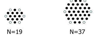
FIG. 6: Cross sections of N=19 and N=37 tori with the lighter circles corresponding to corner filaments. As winding number increases the number of corner filaments always remains 6, so the overall density of corner filaments goes down for large N tori.
