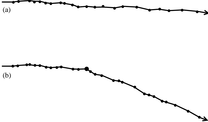
FIG. 2: A depiction of (a) typical multiple scattering (the HO approximation) vs. (b) the rarer case (related to the N=1 approximation) where the total deflection is dominated by a single scattering with unusually large momentum transfer. The scattering angles are all exaggerated in this figure for the sake of visibility. The net angular deflection in both cases is parametrically \ll 1 , and the small-angle scatterings are meant to be significantly smaller than the single larger (but still small) angle scattering in (b).
