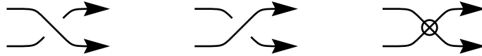
FIGURE 2. The three types of crossing in a virtual knot diagram: real positive (left), real negative (middle) and virtual (right)
