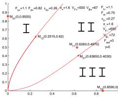
Figure 3: The steady states of system (26). Where the unstable steady states are denoted by "\*", the stable steady states are denoted by "\*". If the initial state  $P_0(x_0, y_0)$  lies in the subdomain I (II or III), then the final state is the stable steady state  $M_{01}$  ( $M_{11}$  or  $M_{10}$ ).)
