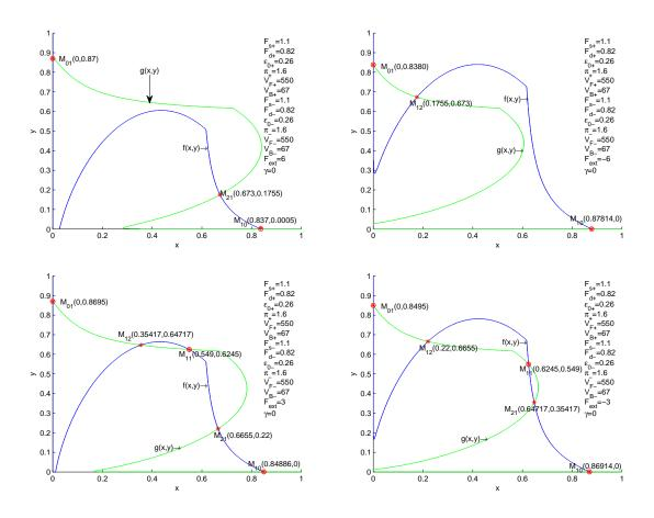
Figure 6: Tug-of-war model with external force  $F_{ext}$ : In this case, the system (26) might have two or three stable steady states.
