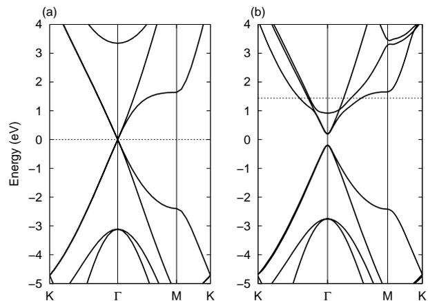
FIG. 1: (a) Band structure of  $C_6^*$ , i.e., graphene described by the unit cell of  $(\sqrt{3} \times \sqrt{3})R30^\circ$  structure. (b) Band structure of  $C_6Li$ . A band gap has opened at the neutrality point, the degenerate bands along the  $\Gamma$ - $K$  direction are split, and a small band gap has opened at  $K$  near the bottom of the figure. Horizontal dashed lines indicate the Fermi levels of the respective systems.
