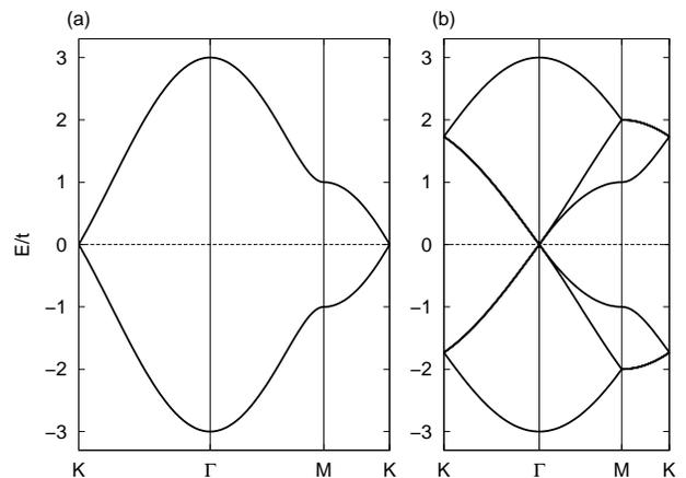
FIG. 3: Band structures of graphene in the Brillouin zones of (a) the  $(1 \times 1)$  structure, and (b) the  $(\sqrt{3} \times \sqrt{3})R30^\circ$  structure.
