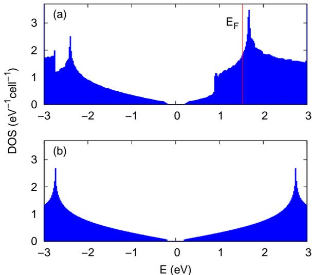
FIG. 5: (Color online) (a) DOS of  $C_6Li$  calculated by DFT code. The vertical red line indicates the position of the Fermi level. (b) The corresponding DOS for graphene calculated within the tight-binding model. The position of Van Hove singularities are displaced relative to the DOS of (a) and the extra densities corresponding to Li atoms are not included in (b).
