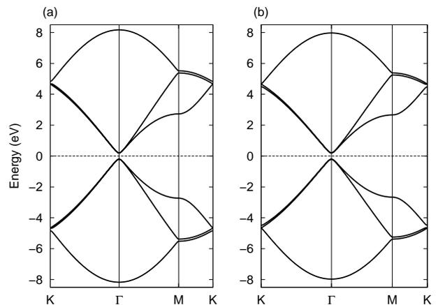
FIG. 4: Band structures of graphene from the TB model with two hopping amplitudes: (a)  $t_1 = 2.79$  eV,  $t_2 = 2.59$  eV, and (b)  $t_1 = 2.59$  eV,  $t_2 = 2.79$  eV. Note that the three-fold degeneracies at  $K$ , e.g., the lower left one, are lifted so that in (a) we have first a non-degenerate level and above it a doubly degenerate level, and in (b) we have just the opposite order of the degenerate and nondegenerate levels.
