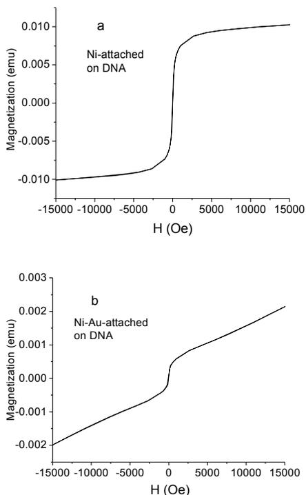
**Figure 3.** Magnetic hysteresis loop of Ni-nanoparticles attached on DNA (a), and Ni<sub>core</sub>-Au<sub>shell</sub>-DNA (b)
