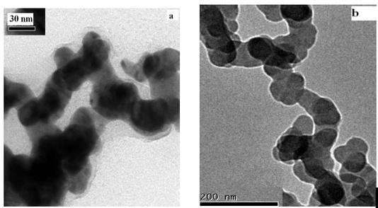
**Figure 2.** TEM images of Ni-nanoparticles attached on DNA (a), and Ni<sub>core</sub>-Au<sub>shell</sub>-DNA (b)
