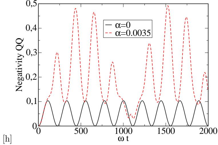
**Figure 2.** (color online) The unitary evolution of the qubit-qubit entanglement as a function of dimensionless time  $\omega t$  and the nonlinearity coefficient  $\alpha$ . The initial state  $|eg0\rangle$ .  $\Omega_i = \omega, \gamma = 0.01\omega$
