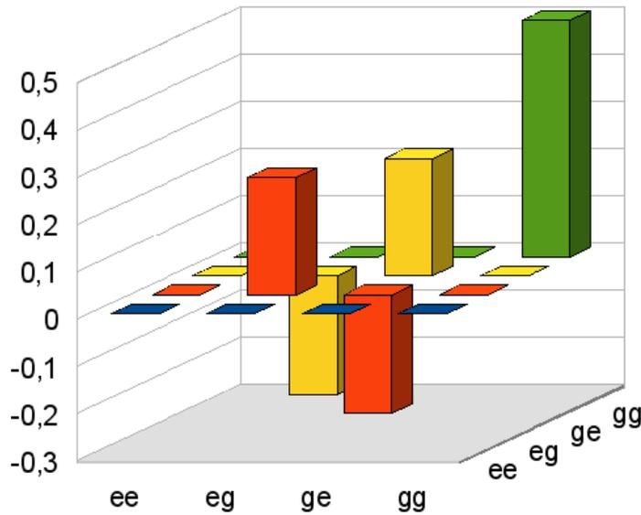
**Figure 7.** (color online) The real part of the qubit-qubit density matrix for the case of the linear resonator and the initial state (9). The matrix is taken at  $\omega t = 111$  for which  $N_{QQ} = 0.104$  (solid line in Fig.2). The imaginary elements of the matrix are of the order of  $10^{-14}$ .
