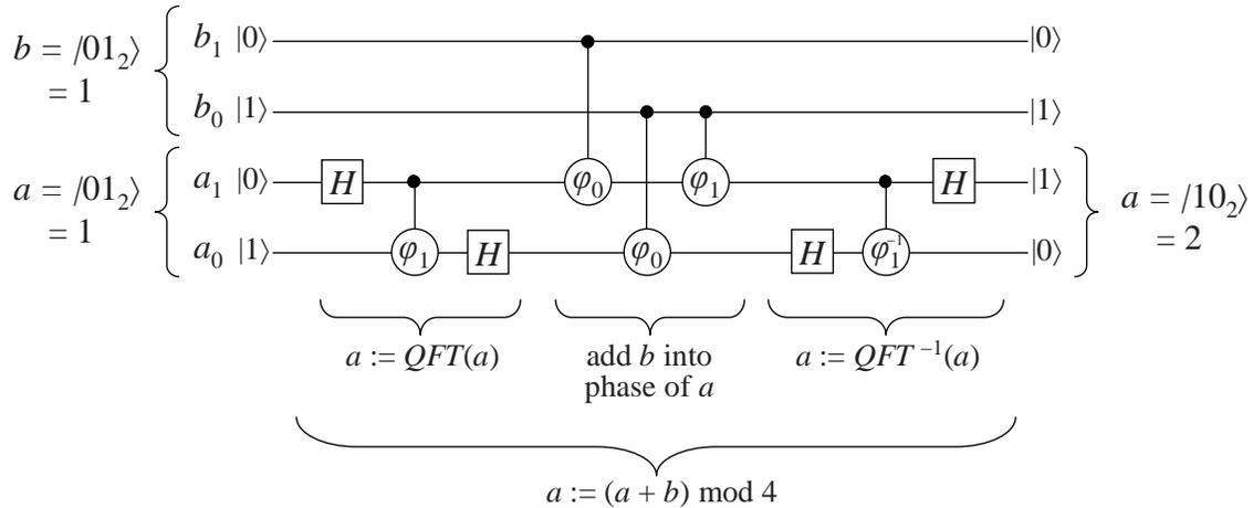
**Figure 1. A simple example quantum circuit.** Uses the quantum Fourier transform (QFT) and its inverse  $QFT^{-1}$  to add two 2-bit input integers in a temporary phase space representation. Here it is computing  $1 + 1 = 2$ .
