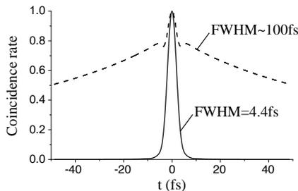
FIG. 3: Solid line:  $|\psi_{\text{pw}}(\vec{x}=0, t)|^2$ , coincidence rate when photon positions are resolved in the near field. Dashed line:  $\int d^2\vec{x} |\psi_{\text{pw}}(\vec{x}, t)|^2$ , coincidence rate measured without resolving photon positions
