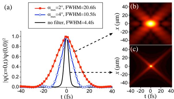
FIG. 4: (Color online) Effect of spatial filtering on the X-entanglement: (a) Temporal correlation peak  $|\psi_{\text{pw}}(0, t)|^2$  in the presence of a spatial filter, that cuts the angular spectrum at an angle  $\alpha_{\text{max}}$ . The two insets show the full X-correlation for  $\alpha_{\text{max}} = 2^\circ$  (b), and in the absence of any filter (c).
