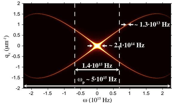
FIG. 2: (Color online) Plot of  $|V(q_x, \omega)|$ , showing the phase matching curve. The dashed vertical lines show the frequency bandwidth selected by the filter and the arrows indicate the different bandwidths involved (same parameters as in Fig.1).
