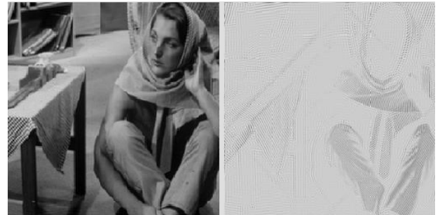
Figure 2: The representation result in last iteration of proposed algorithm for the Barbara image. (left) Output of curvelet transform with six resolution levels. (right) Output of local-DCT representation with a block size 32 \times 32 .
