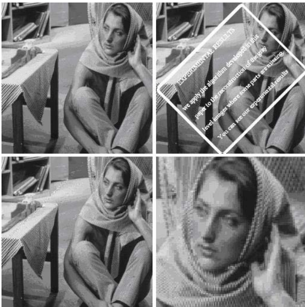
Figure 2: The reconstruction of the masked image. (top left) Original image. (top right) The target regions are masked in white. (bottom left) Region filling via the proposed inpainting algorithm. (bottom right) The result of our algorithm around Barbara's eyes.
