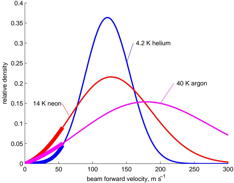
FIG. 3: Theoretical energy spectrum for hydrodynamic beams using 4.2 K Helium, 14 K Neon, or 40 K Argon as a buffer gas. The portion of the distribution with an energy of less than 4K is shown in bold. Neon is clearly an attractive choice for experiments interested in maximizing the flux of very cold atoms or molecules.
