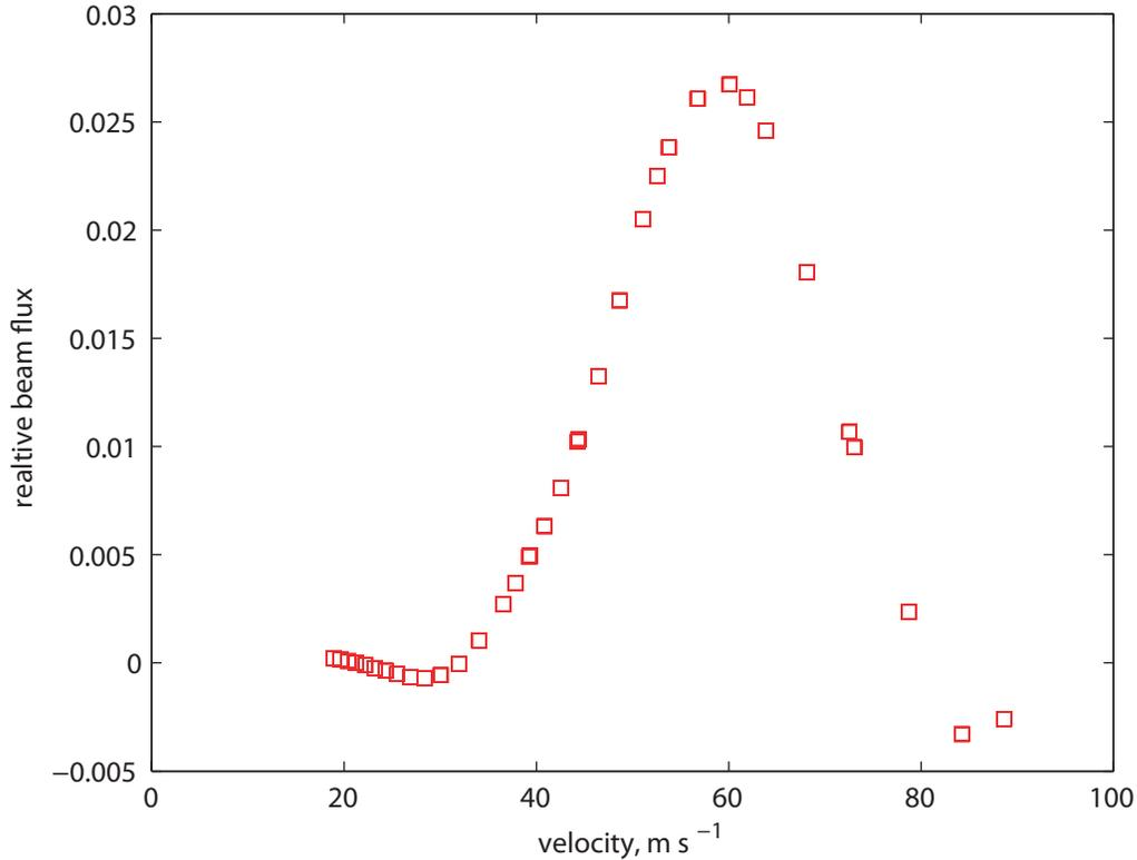
FIG. 6: Velocity distribution at the output of a 70 cm long electrostatic guide with a bend radius of 8 cm. The output of this guide is completely separated from the neon buffer gas, and represents a pure, state-selected, low energy beam. This data represents  $3 \times 10^8$  ND<sub>3</sub> molecules s<sup>-1</sup>, with a mean energy of about 4 K.
