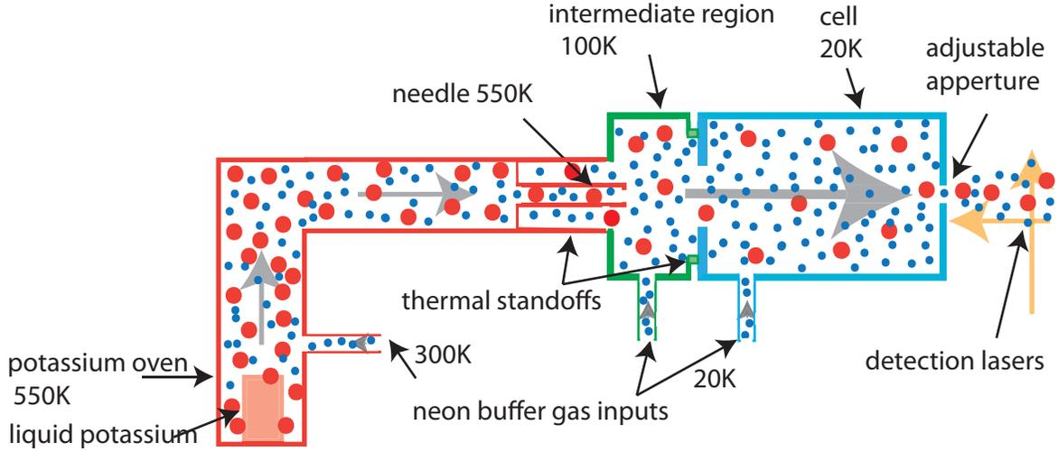
FIG. 1: Overview of apparatus. An oven supplies a hot (550K) mixture of potassium and neon that flows through an intermediate region (100K) to a cold tube “cell”. (15K). The oven, intermediate plate, and cell are separated by thermal standoffs to reduce heat loads. A cold beam of potassium and neon exits an adjustable aperture on the far side of the cell where its characteristics are measured by absorption spectroscopy.
