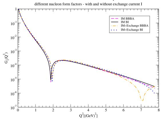
FIG. 7: (color online) Deuteron form factor  $G_1(Q^2)$ ; ; different nucleon form factors with and without exchange current I
