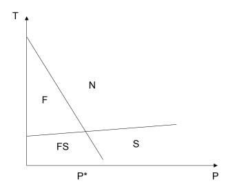
**FIGURE 1.** The schematic pressure-temperature phase diagram of superconducting UCoGe. Here, N is the normal paramagnet phase, F is the ferromagnet phase, S is the paramagnet superconducting phase, S is the multi-domain ferromagnet superconducting phase. All the lines are the lines of the second-order phase transitions.
