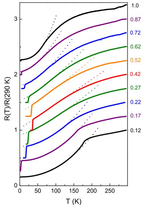
FIG. 2: (Color online) Resistivity of  $K_xSr_{1-x}Fe_2As_2$  vs. temperature for  $0 \leq x \leq 1$ . For clarity different curves are vertically offset by 0.25 units. The labels mark the values of  $x$ . The dotted lines show the fit to a power law,  $\rho(T) = \rho_0 + AT^n$  with the exponents  $n$  shown in Fig. 3.
