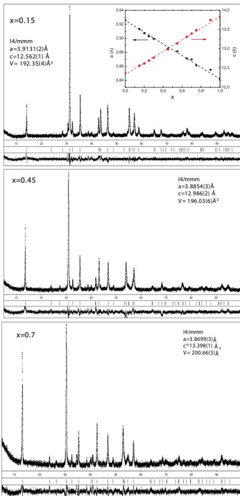
FIG. 1: (Color online) Selected X-ray spectra of the system  $K_xSr_{1-x}Fe_2As_2$  for  $x=0.15, 0.45, 0.7$ . The inset shows the change of lattice parameters  $a$  and  $c$  with  $x$ .
