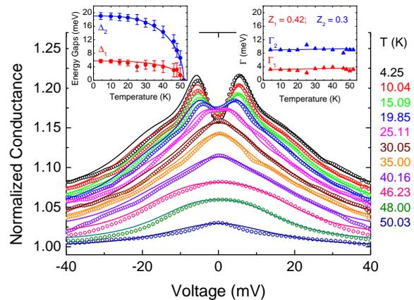
FIG. 3: (color online) Temperature dependence of the normalized conductance curves (symbols) together with their relevant two-gap BTK fits (lines). The curves are vertically shifted for clarity. The raw data are those shown in Fig. 1 and the insets show the temperature dependency of the gaps ( $\Delta_1$  and  $\Delta_2$ ) and of the broadening parameters ( $\Gamma_1$  and  $\Gamma_2$ ) given by the two-gap fit.
