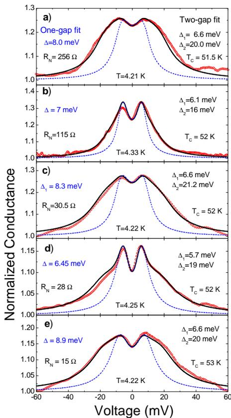
FIG. 2: (color online) (a) to (e): normalized conductance curves (symbols) at 4.2 K in  $\text{SmFeAsO}_{0.8}\text{F}_{0.2}$ . The contact resistance,  $R_N$ , decreases from top to bottom. The curves are reported together with their relevant one-gap (dash lines) and two-gap (solid lines) BTK fits. The gap values are indicated on the left (single-gap fit) and on the right (two-gap fit).
