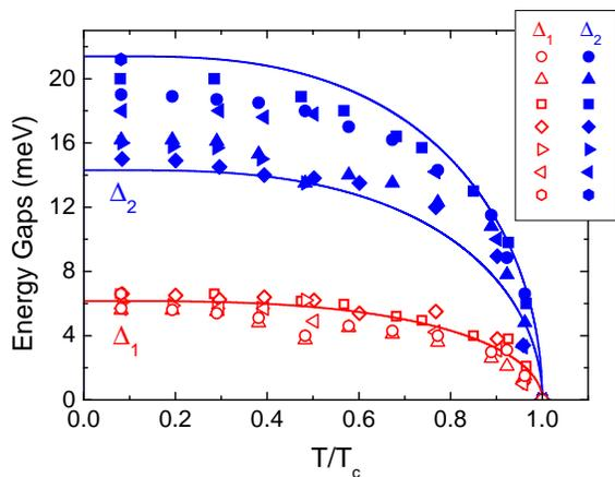
FIG. 4: (color online) Temperature dependence of the gaps  $\Delta_1$  (open symbols) and  $\Delta_2$  (full symbols) as extracted from the two-gap fit of the conductance curves. Lines are BCS-like curves. Details are in the text.
