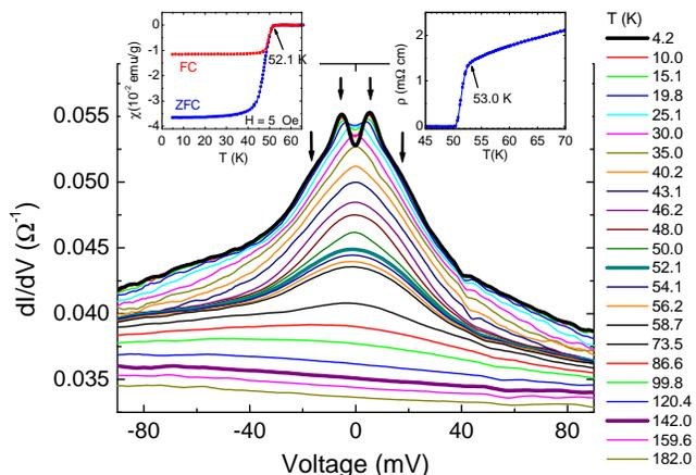
FIG. 1: (color online) Temperature dependence of the raw conductance curves of a point contact with  $T_c \sim 52$  K. The low-temperature curve (upper thick line) features two peaks and two shoulders (indicated by arrows) related to  $\Delta_1$  and  $\Delta_2$ , respectively. The curve at  $T_c$  (middle thick line) has a hump-like shape which flattens at  $\sim 140$  K (lower thick line). Insets show the resistivity and dc susceptibility of the sample.
