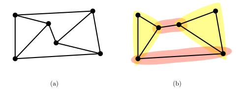
FIGURE 1. Laman graphs and rigid components: (a) a Laman graph on n = 6 vertices; (b) a flexible graph with its rigid components indicated.
