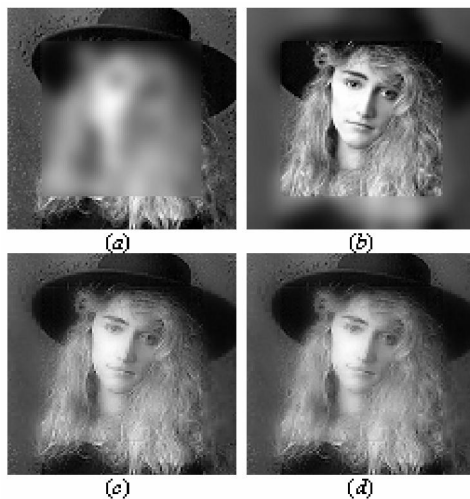
Fig. 7: Results for Hoed image a) Middle part blurred image b) Corner part blurred image c) Result of DWT algorithm d) Result of DWPT algorithm
