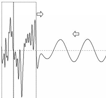
FIG. 6: The  $z$ -component of the electric field along the  $x$ -axis (at  $y = 0$ ), showing the incident source pulse overlapped with the first two consecutive cycles of the reflected radiation. Both the cycles exhibit presence of high harmonics. The second cycle (left) is compressed in comparison with the first cycle because the mirror velocity is increasing, which results in the increase of the compression factor according to Eq. (3).
