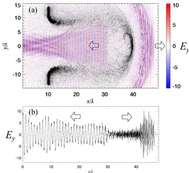
FIG. 5: (a) The  $z$ -component of the electric field, representing the source pulse, and the ion density (black). (b) The profile of the  $z$ -component of the electric field along the  $x$ -axis at  $y = 0$ . Both the frames for  $t = 37 \times 2\pi/\omega$ . In the frame (a), strongly jagged distribution is not seen in the colorscale in the interval  $40 < x/\lambda < 42$  due to the sampling (the wavelength is smaller than the image pixel).
