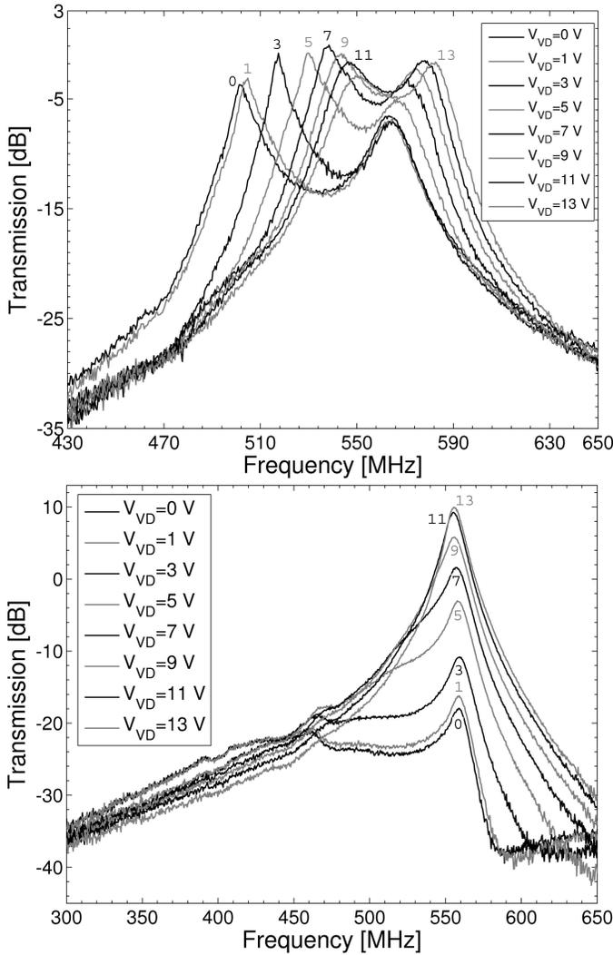
FIG. 2: Transmission vs. frequency curves obtained at  $\Phi_1 = 0.475\Phi_0$  with a network analyzer at 0.309K (-99dBm incoming power) with the MSA 'ON' i.e. optimally biased to have the largest respectively positive or negative transfer function (upper or lower figure). The voltage  $V_{VD}$  across the varactor diode placed at the end of the microstrip is varied. Calibration was performed with the PC board illustrated in the inset of fig. 1 replaced by a short transmission line.
