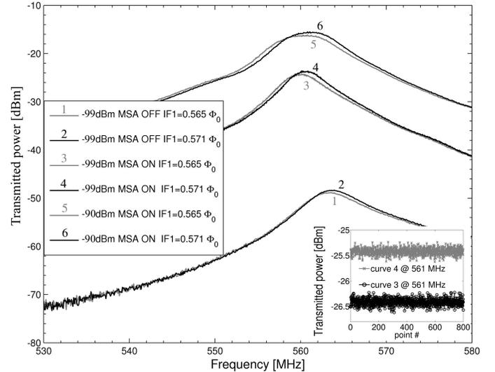
FIG. 3: Transmitted power vs. frequency measured with a spectrum analyzer for a couple of input flux values ( $6m\Phi_0$  apart) with the MSA OFF or ON with an incoming power of -99 or -90dBm. Inset: power spectrum at 561MHz for curve 3 and 4.
