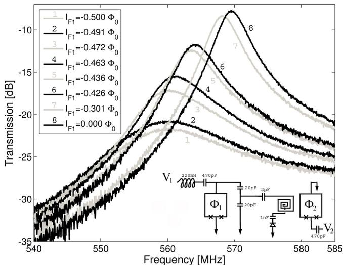
FIG. 1: Transmission vs frequency curves obtained at 0.309K and with the MSA OFF, for different input flux in the tank circuit Squid ( $I_{F1}$ ). After the attenuators, the incoming power is -99dBm. Inset is a schema of the low temperature part of the readout circuit.
