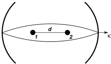
FIG. 1: Schematic diagram of the system. Two qubits are trapped in a high- $Q$  cavity and are symmetrically located about the antinode of the standing-wave cavity mode.
