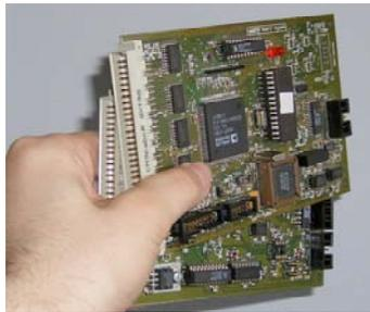
**Fig. 4.4.** The realized KLJN network unit with a pair of KLJN communicators [7]. The computer chip version can be much simpler because of the very short cable distances in the computer providing idealistic conditions to approach the theoretical limits of performance.
